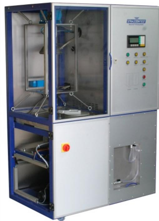
By reason of its compact and closed design, the new type 520 perfectly prevents the emission of solvents. Aggregates and filler will be dried within the system and the solvent, which condenses during the drying process, is kept in the machine. This serves best protection of the operating personnel and the environment, performed with the same analysis method, which is well-proved within more than 20 years now.
