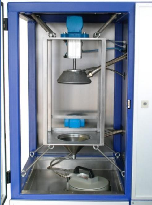
The function of the new binder extraction machine is as described above. Just one detail is essentially improved: The sieve set is shaken in three dimensions now, while shaken in two directions former. So the wash-out effect by means of the solvent is more efficient and the effect of obstructing the sieves during the wash-out process is almost eliminated.
