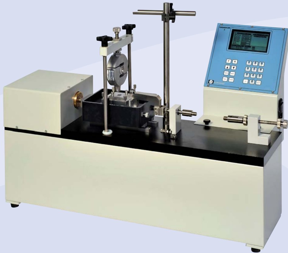
VJT 2571 ShearSCAN 2 Pneumatic Direct/Residual Shear Box
